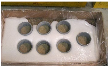
InstaGrout flows and expands after 20 minutes
