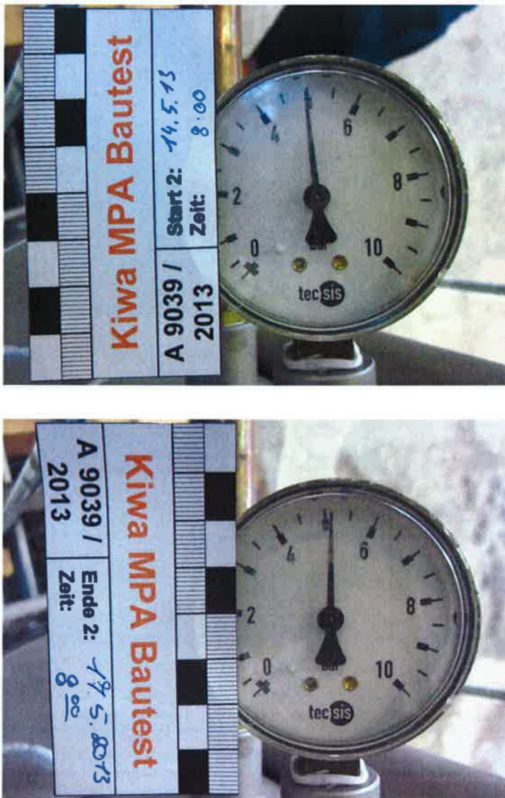
Figure 6: Pressure leak test with the water-filled pressure bell at room temperature (top: Pressure gauge reading at start of the test on 05/14/2013 at 08:00; bottom: Pressure gauge reading following the end of the test on 05/17/2013 at 08:00)
