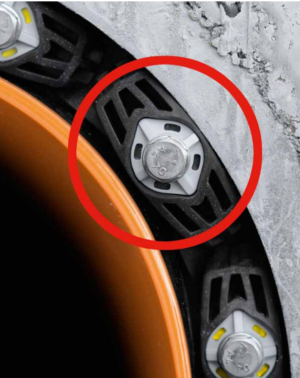
PGKD 400 with one segment not tightened – installation error immediately detected
